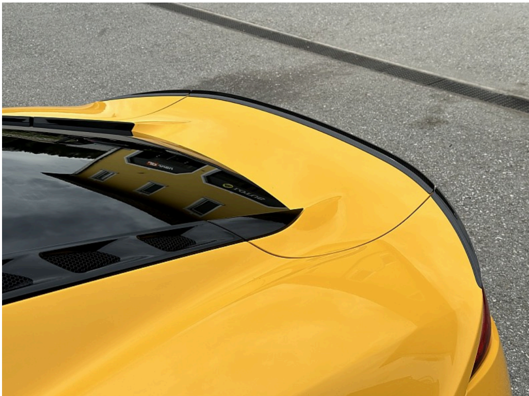
Fig 3: JUBU carbon gurney ready installed.
