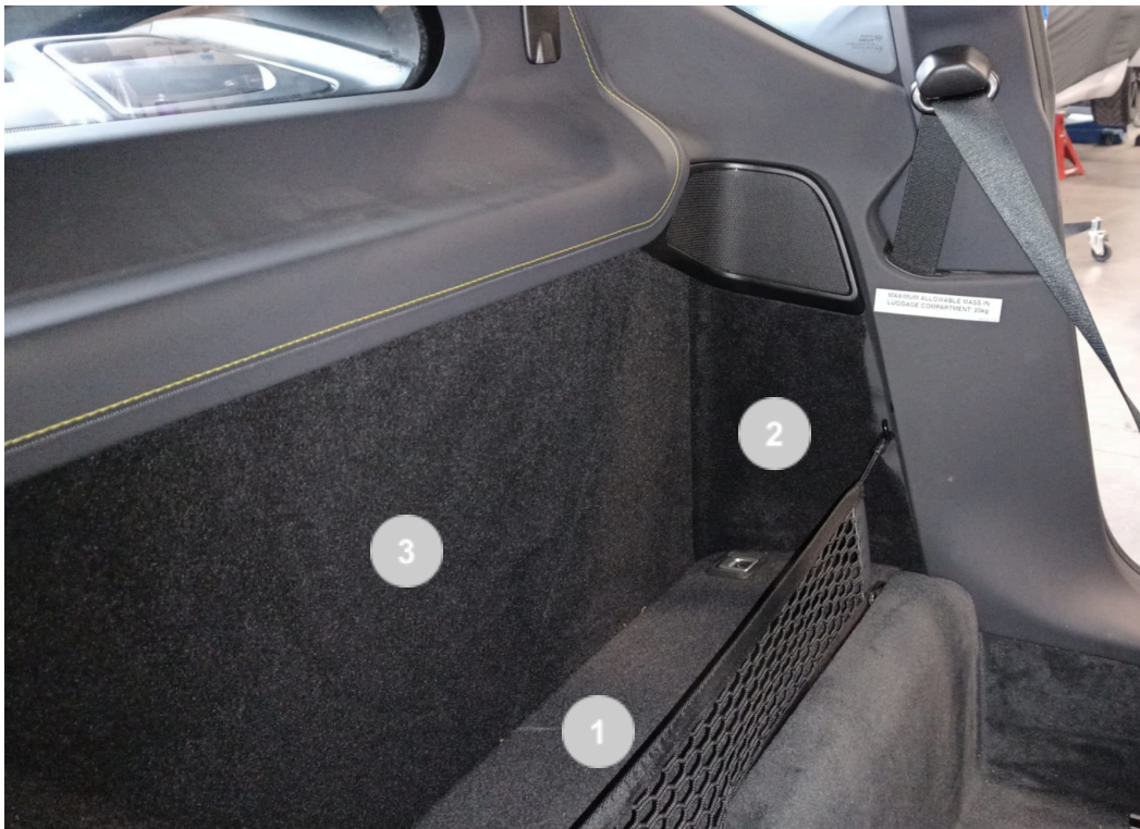
Fig 2: Uninstall the rear interior panels.
