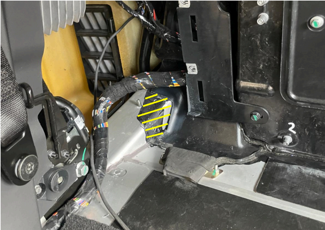
Fig 5: Trim the lower ends of the rear bulkhead II
