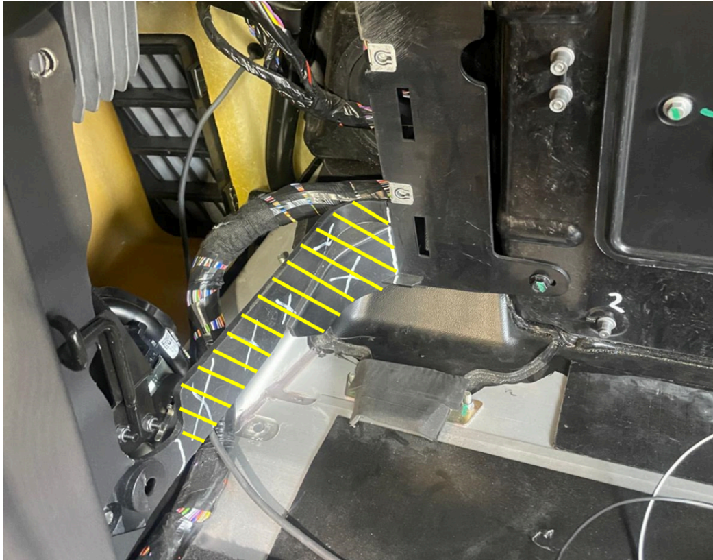
Fig 3: Trimming the plastic brackets in the rear corners.
