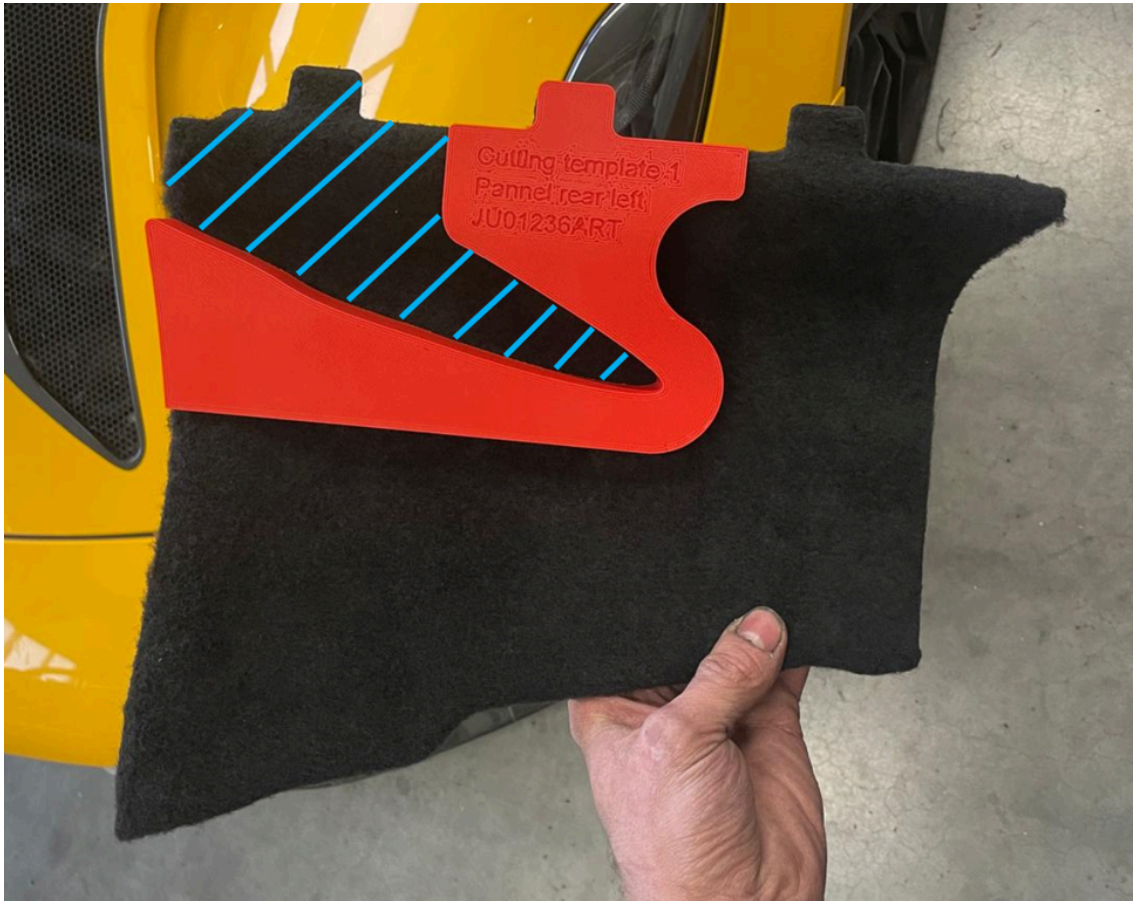
Fig 9: Trimming the carpet panels for the rear corners.
